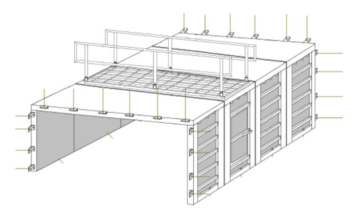
This design is supplied in unrated, 2 PSI rated and 5 PSI rated and can be fitted with man access doors if required.
